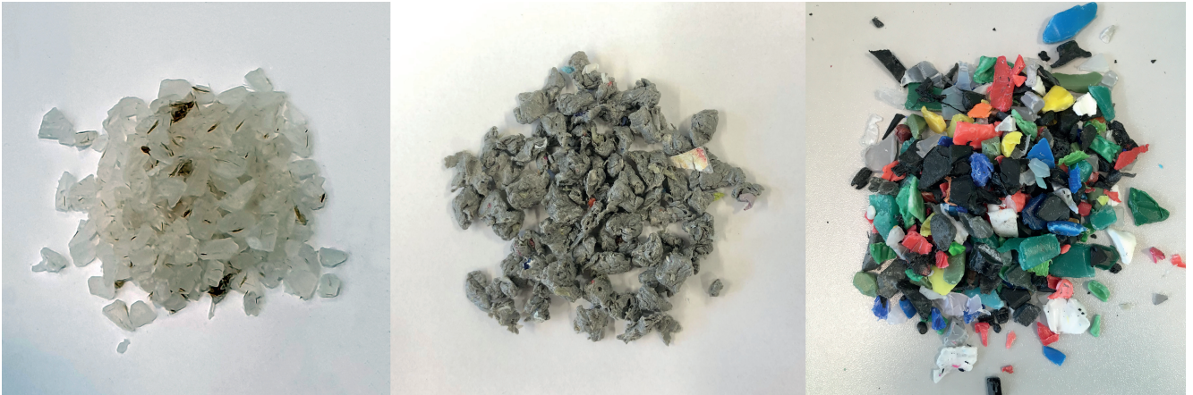
Fig. 1. The tests were carried out on three different materials: pellets of virgin PP (left), PP agglomerate obtained from post-consumer film (center) and regrind obtained from HDPE beverage closures (right). © Engel
